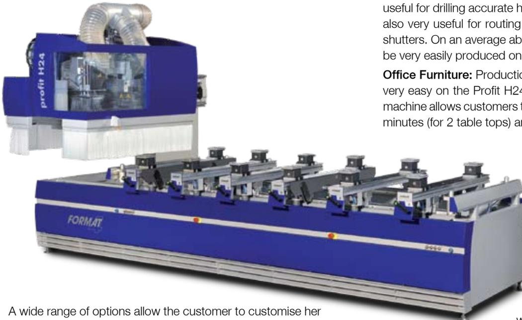
**Kitchen Production:** A Profit H20 (with consoles) can be very useful for drilling accurate holes for kitchen carcasses. It can be also very useful for routing out profiles for membrane pressed shutters. On an average about 80 – 100 carcasses per day can be very easily produced on the Profit H20.
