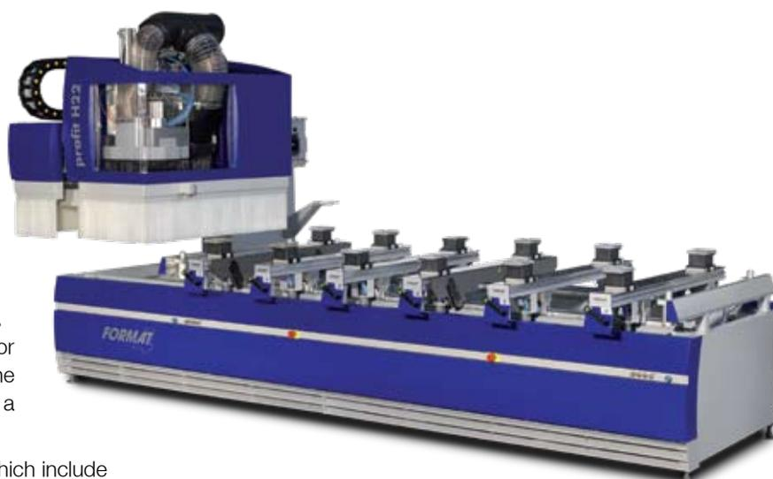
(X, Y and Z). A 4th axis (C-axis), which is also fully interpolating, can also be added. The C-axis increases the possibilities for the customer, allowing her to use a wide range of aggregates.
