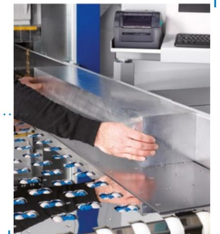
Angular table with air cushions and rollers on all sides for energy-saving material handling.
