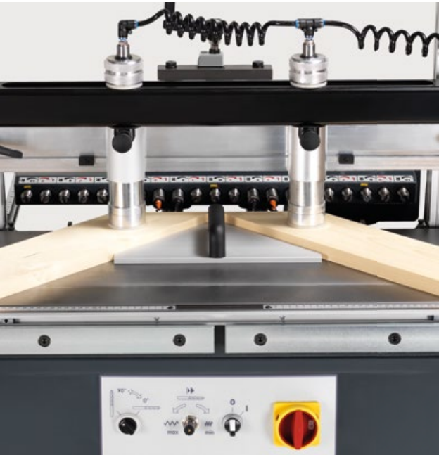
Straight or at an angle The 90° fence and the 45° mitre fence offer comfort and precision with every application.
