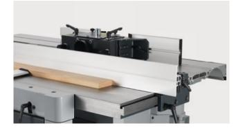
The Felder planer fence The planer fence can be tilted to any position from 90° to  $45^{\circ}$ . There is an end stop at both the 90° and  $45^{\circ}$ positions.
