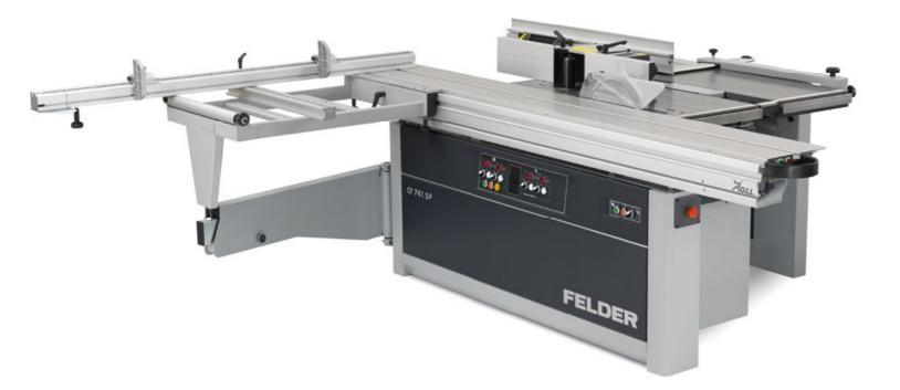
Everything you need for perfect woodworking results in just two and a half square meters: the Felder CF 741 woodworking system combines the advantages of five stand-alone machines and brings high performance, precision and the shortest change-over times to every workshop. Planing, shaping, cutting and drilling a top quality workshop in one machine. The operating comfort is increased even further with the Professional package, ensuring simple processing of larger workpieces.
