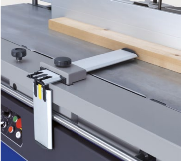
Comfort jointer guard Maximum work safety and unparalleled ease of use: The space-saving dressing guard integrated into the machine column stabilizes the workpiece during dressing and joining operations.
