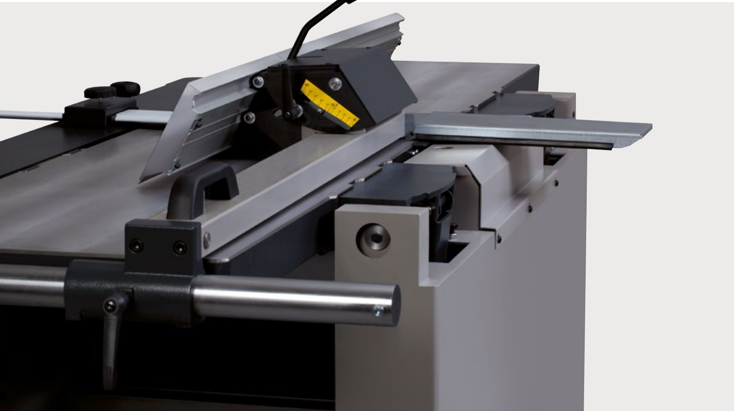
The Felder planer fence The planer fence: A masterpiece of space saving design that ensures stability and precision! The planer fence can be tilted to any position from 90° to 45°. There is an end stop at both the 90° and 45° positions.
