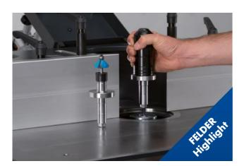
MF Spindle shaft quick change system Without losing any settings, just a few turns of your hand allows you to swap spindles of varying diameters.
