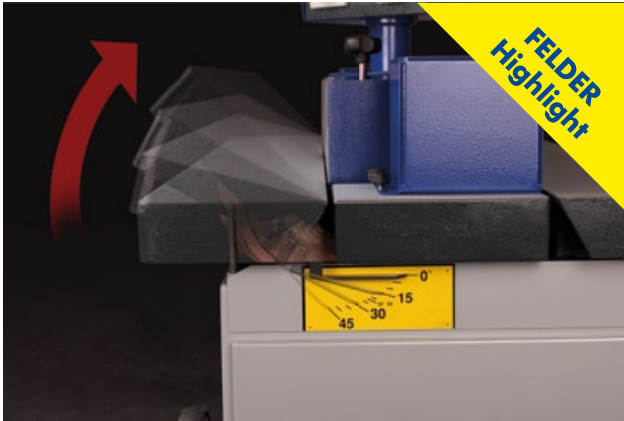
Sanding table The sanding table may be tilted continuously between 90° and 45° for angular sanding work.
