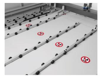
**Roller track** The roller track supports the material pusher transport of panels and guarantees a precise feed of the panel material to the cutting line.
