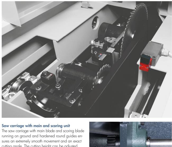
cutting angle. The cutting height can be adjusted manually, pneumatically or using electro-motors.
