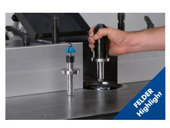
MF Spindle shaft quick change system
