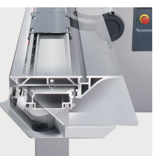
**Locking pin**Angles at 5 degree intervals and at 22.5° can be cut with the help of the index locating pins.
