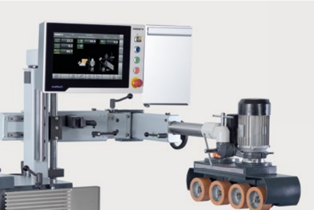
Electrical height-adjustable feed support The height of the power feeder is set via the self-explanatory e-motion control on the 15" touchscreen. The infeed unit positions itself to the selected setting value utilizing an electric motor, and the integrated automatic on/off switch ensures absolute ease of operation. For set-up work, the feeder is swivelled completely out of the working area.
