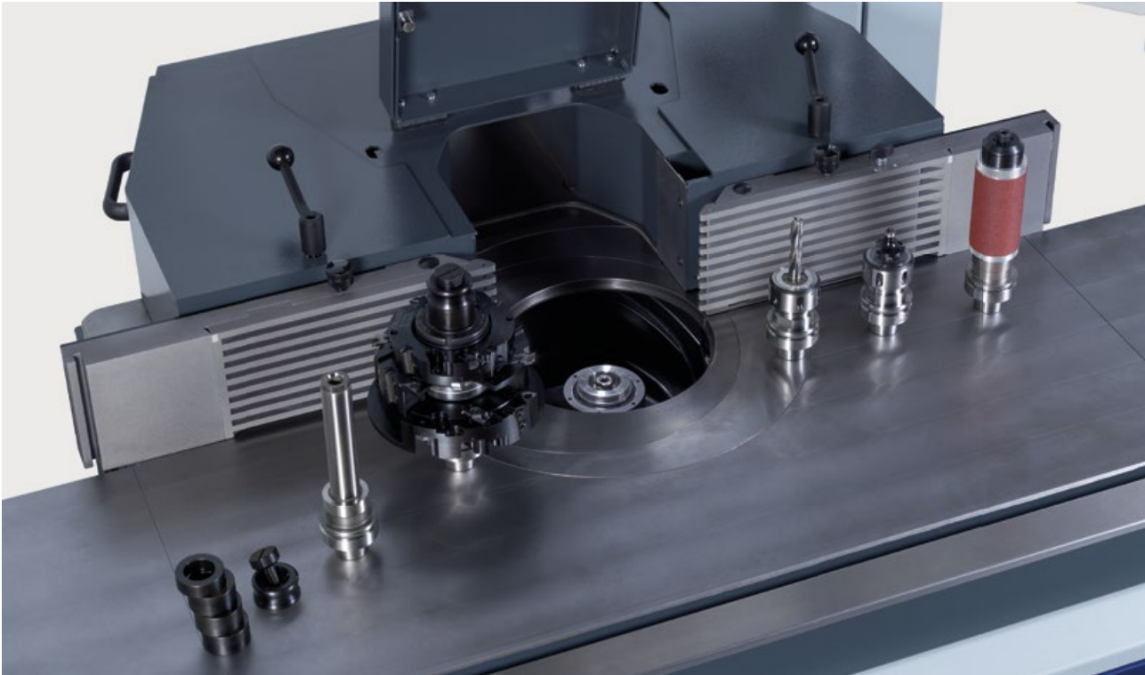
Quick-change cutter arbor system HSK F63 The profil 92 electro-spindle cutter arbor is equipped with an HSK F63 quick-change tool system with pneumatic clamping and an air jet nozzle system for cleaning the contact surfaces. In a matter of seconds, cutter arbors with pre-mounted cutter tools can be changed for series milling work. The HSK F63 quick-change cutter arbor system also ensures maximum flexibility and efficiency when using different cutter arbor diameters or when using shaft cutters with collet chucks.
