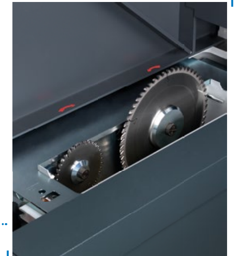
Saw carriage with main and scoring unit, high precision and wear-free guiding system.
