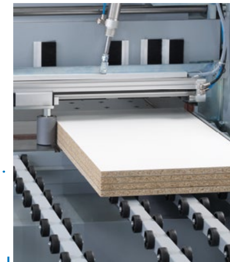
Angle pressing device for a gentle and precise alignment of the panels.
