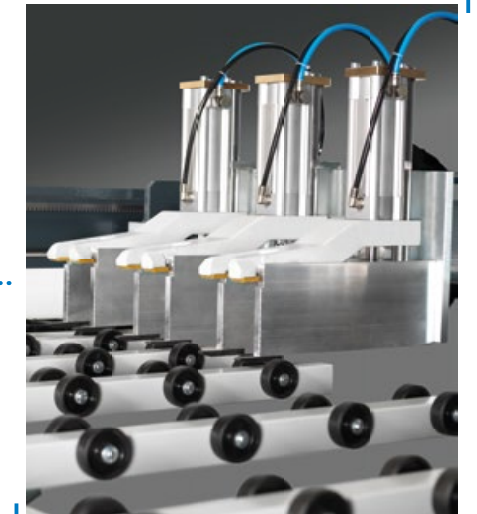
Double-finger Package clamp with variable pressure setting.
