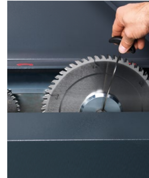
ProLock® EasyFix saw blade quick-change system guarantees the shortest setup times.
