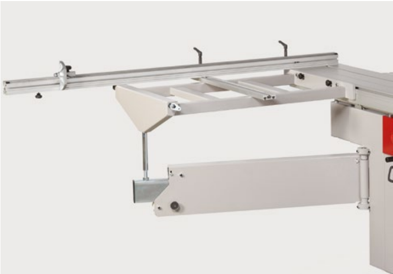
Outrigger table for heavy workpieces The outrigger table provides additional surface support and precision when processing large dimensioned and heavy workpieces. In combination with a 900 or 1300 aluminum crosscut fence and the crosscut extension your Hammer with outrigger table becomes a complete, large panel saw.
