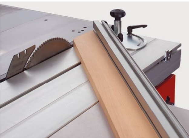
Crosscut fence for precise mitre cuts Adjustable to any position between +45° and -45°, the crosscut fence ensures precise angled and mitre cuts. A scale integrated into the aluminum sliding table makes it easy to set precisely. The end stop for the 90° position guarantees absolute precision with repeat settings. The scale on the 35.43” long aluminum crosscut fence is angled towards the operator and makes it easy to comfortably read the exact setting. In combination with the crosscut stop with integrated magnifying glass, highly precise settings and as such absolutely exact results are guaranteed.
