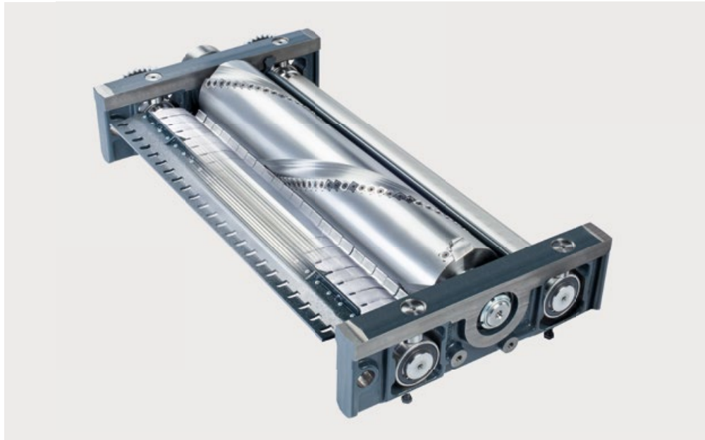
Stability for high performance The solid cast iron cutterblock housing is built for heavy duty work. The serrated steel infeed roller and the micro-serrated steel outfeed roller ensure a perfect workpiece transport. Both steel rollers are large dimensioned and non-wearing.
