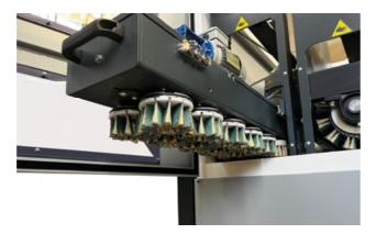
**Quick change system for grinding inserts** The grinding inserts on the longitudinal and disc brushes can be exchanged quickly and easily and reduce any set-up times enormously.
