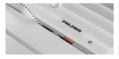
**Safety made visible – Scoring unit operation display** A red LED strip immediately signals the operation of the scoring unit and offers even more working safety.
