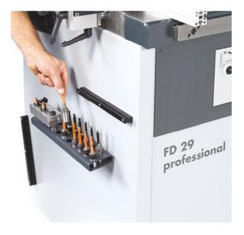
**Everything in its place**Holders for the side fences, fence extensions and two tool holders each with the capacity for 21 tools, ensures that all equipment required is always at hand.
