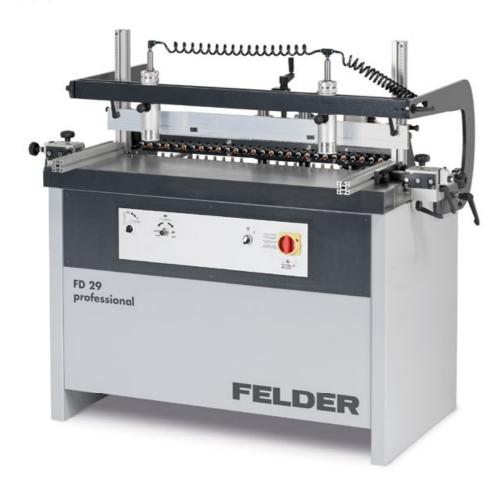
Maximum precision when dowel boring with the Felder FD 29 professional. With 29 high quality drilling spindles at a distance of 32 mm, for drill bits with a diameter of maximum 35 mm, exact dowel and line boring holes are guaranteed. The welded chassis in combination with the solid cast iron table, rigid side and longitudinal stops, as well as pneumatic workpiece holders and ergonomically designed operating elements ensure that the FD 29 professional, is a dowel boring machine of the top class.
