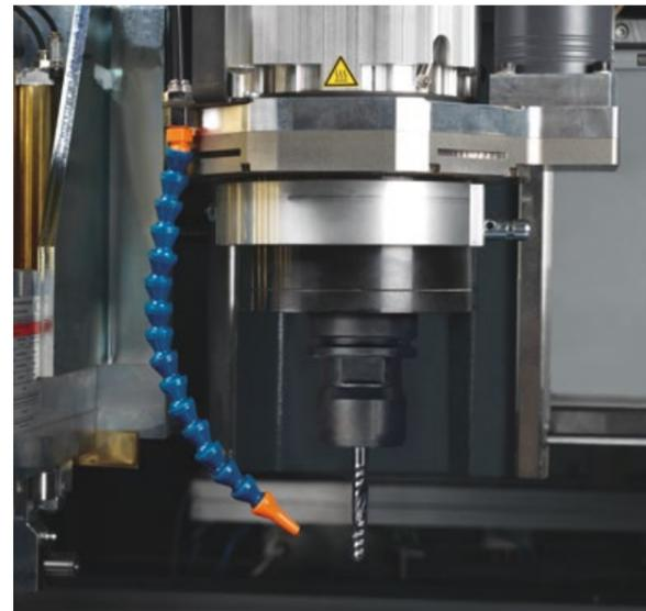
**Adjustable, controlled compressed air and cold air jets (21.31 c-tech)**
