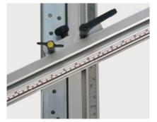
Angles at 5 degree intervals and at 22.5° can be cut with the help of the index locating pins.
