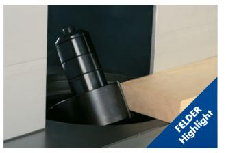
**Moulder spindle tilt 90°–45°** The Felder rearward tilting Spindle is the correct way for easy and safe operation:
