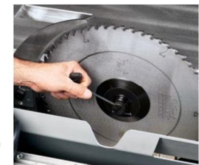
**Simple, safe & quick – "Quick-lock" saw blade clamping**
