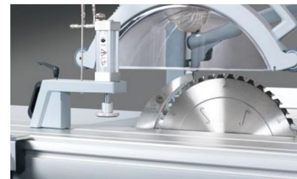
**Pneumatic workpiece holder**
