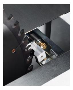
Minimum quantity lubrication system (MMS) integrated in the saw carriage for the main saw blade.
