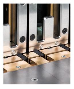
Feeding table with pneumatic pressure roller for exact angular cuts even of long components.
