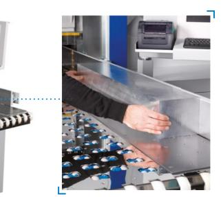
Angular table with air cushions and rollers on all sides for energy-saving material handling.
