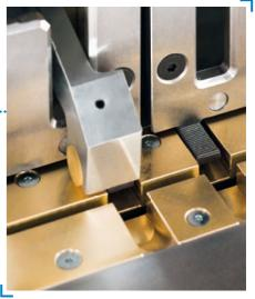
Interchangeable cutting lips made of nonferrous metal.
