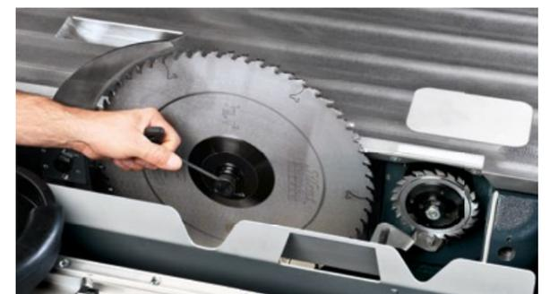
**Simple, safe & quick – "Quick-lock" saw blade clamping**
