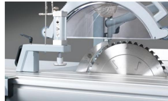
**Pneumatic workpiece holder**
