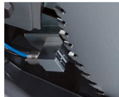
**Spraying unit for processing non-ferrous metals and plastics**
