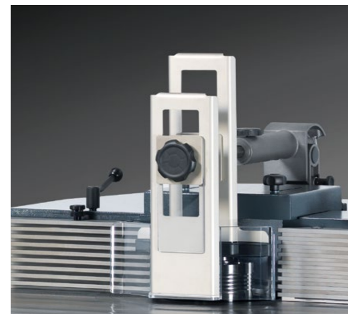
Centrex spindle moulder guard The high-quality, flexibly adjustable Centrex moulder guard, which presses the workpiece against the moulding table and fence, ensures safety and comfort during manual milling work. When using a power feeder, the Centrex moulder guard is simply moved out of the working area.
