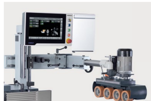
Electrical height-adjustable feed support The height of the power feeder is set via the self-explanatory e-motion control on the 15" touchscreen. The infeed unit positions itself to the selected setting value by means of an electric motor, and the integrated automatic on/off switch ensures absolute ease of operation. For set-up work, the feeder is swivelled completely out of the working area.
