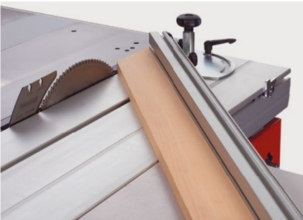
Crosscut fence for precise mitre cuts Adjustable to any position between +45° and -45°, the crosscut fence ensures precise angled and mitre cuts. A scale integrated into the aluminium sliding table makes it easy to set precisely. The end stop for the 90° position guarantees absolute precision with repeat settings. The scale on the 900 mm long aluminium crosscut fence is angled towards the operator and makes it easy to comfortably read the exact setting. In combination with the crosscut stop with integrated magnifying glass, highly precise settings and as such absolutely exact results are guaranteed.
