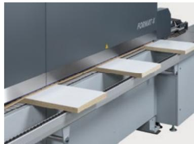
**Variable feed speed in 1 m/min increments for 12–25 m/min (optional)**
