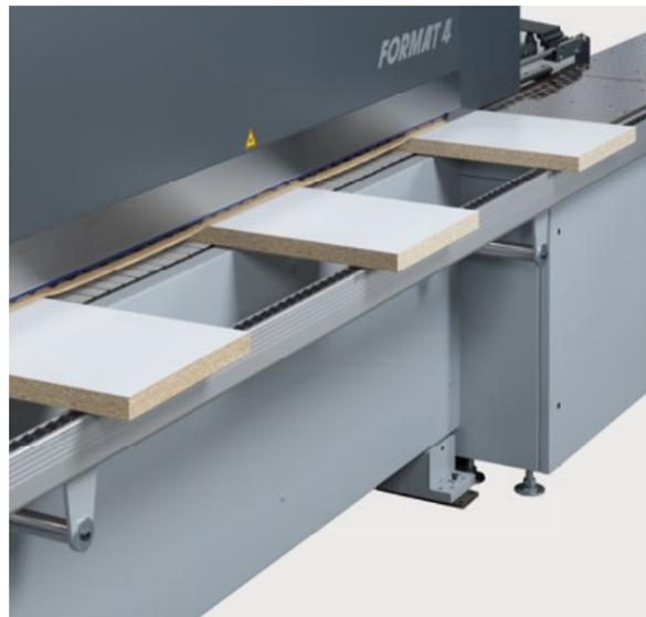
**variable feed speed in 1 m/min increments for 12–20 m/min (optional)**
