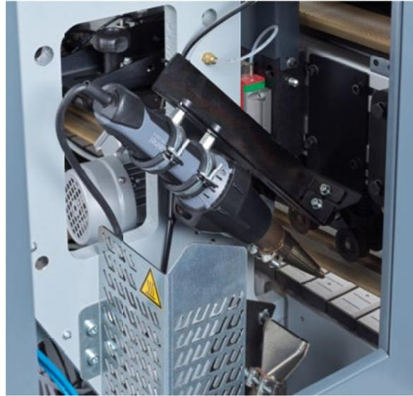
**Hot air blow dryer at the machine outfeed (optional)**
