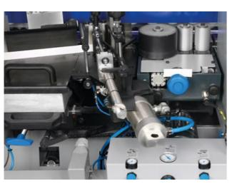
**Pressure zone – Practically invisible glue-joint** Solid in its design, the first operation controlled motor driven roller presses the edge material on to the workpiece. The application control ensures that there can be no smearing of glue or movement of the edge material whilst processing. Both the conical pressure rollers close the glue joint above and below.
