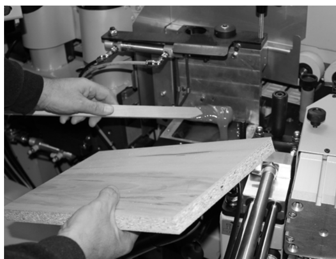
Fig. 10-9.1: Replacing the burnt glue
