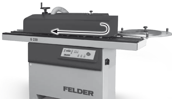
Fig. 2-12: Direction of the Motor rotation
