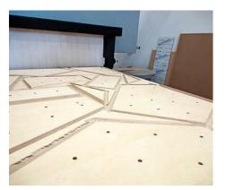
*I* The new nesting process saves up to 15% in material compared with the former process.
