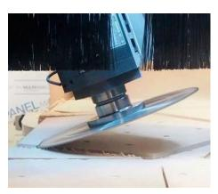
*I* Spectacular: The saw blade is also used as part of the nesting process on the Format-4-CNC machine.
