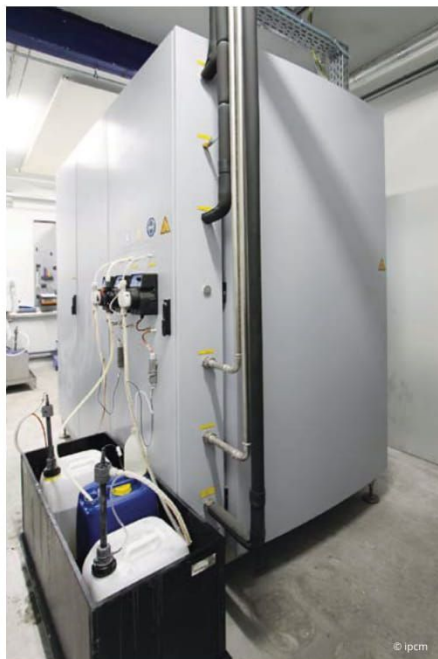
The atmospheric-pressure mechanical compression evaporator manufactured by MKR Metzger.
