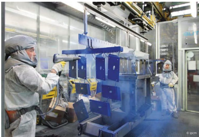
The powder application booth of the coating line for small and medium-sized parts.
