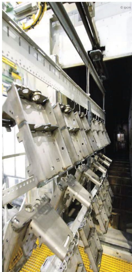
The 5-stage pre-treatment system of the coating line for small and medium-sized parts.
