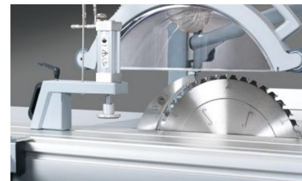
**Pneumatic workpiece holder**
