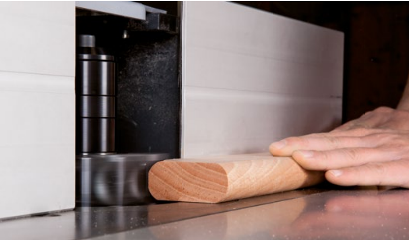
moulder spindle The standard: Moulder spindle-Ø 30 mm for standard moulding tools. Ideal for all „classic“ moulding work.
