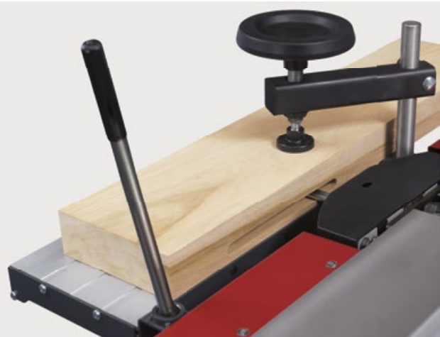
The Mortising Unit The mortising unit is mounted to the planer side.
