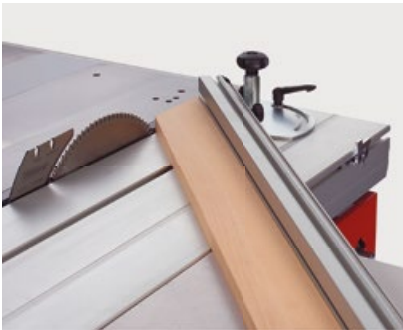
Crosscut fence for precise mitre cuts Adjustable to any position between +45° and -45°, the crosscut fence ensures precise angled and mitre cuts. A scale integrated into the aluminum sliding table makes it easy to set precisely. The end stop for the 90° position guarantees absolute precision with repeat settings. The scale on the 35 7/16" (900 mm) long aluminium crosscut fence is angled towards the operator, making it easy to read the exact setting comfortably. In combination with the crosscut stop with integrated magnifying glass, highly precise settings and as such absolutely exact results are guaranteed.
