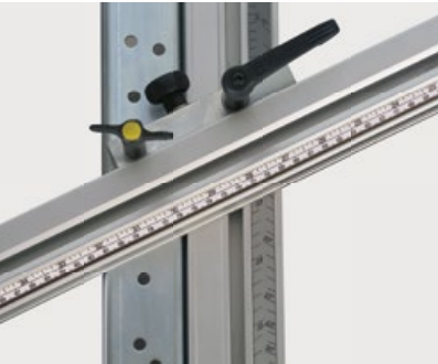
Locking pin Angles at 5 degree intervals and at 22.5° can be cut with the help of the index locating pins.
