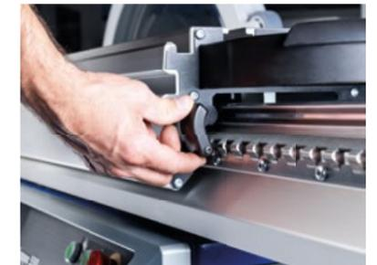
**Fix in every position – Multiple position locking of the sliding table**
