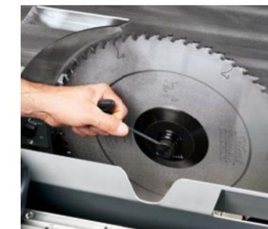
**Simple, safe & quick – "Quick-lock" saw blade clamping**
