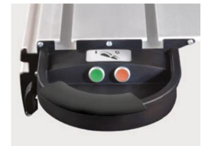
**Remote "ON"-switch on Format sliding table.**
