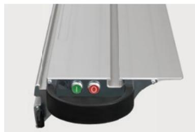
**Remote ON switch on sliding table**
