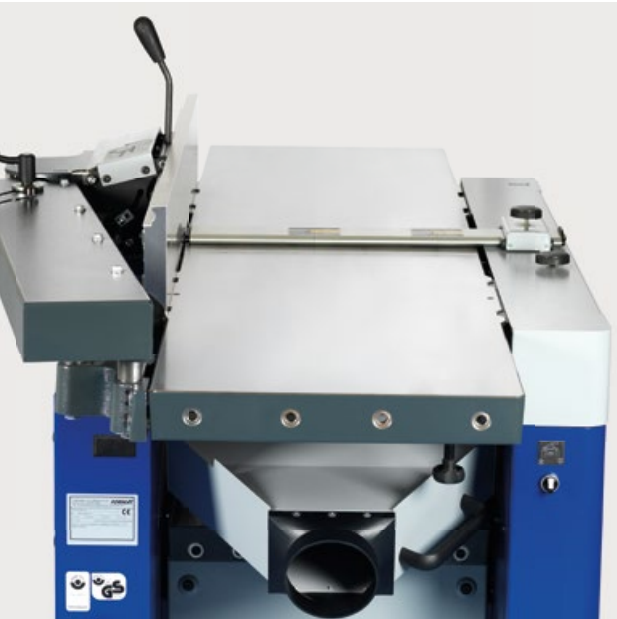
Stability, precision and space saving with the Format4 planing fence A masterpiece of stability, precision and space saving design – the innovative parallelogram system on the Format4 planing fence allows you to be able to position your machine directly next to the workshop wall, without restricting the planing width. The jointer fence can be tilted to any position between 90°–45°, the jointer fence will always remain flush with the jointing table.
