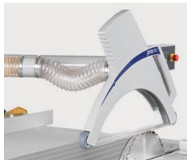
**Overhead saw guard with below table extraction**
