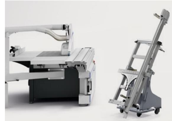
**Transport and mounting unit for outrigger table**
