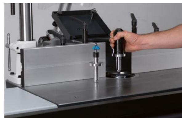
**MF Spindle shaft quick change system**
