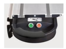
On and off switch on the sliding table
