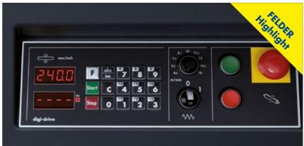
The programmable "Digi-Drive" planing table control makes it possible to enter the planing height using the numeric keypad and the planing bed positions itself automatically and precisely. Two integrated LED displays show the current target and actual values. To optimise production you can save incremental measurements and individual thicknessing table positions.
